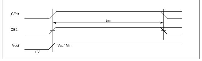
Note : The tothe specifies after Vccr reaches specified minimum level and applicable both  $\overline{CE}$ 1r and CE2r.
